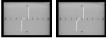
The curved portion of the zener diode signature on the right indicates slow biasing
