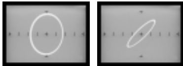
The signature of the capacitor on the right is showing resistance indicating current leakage
