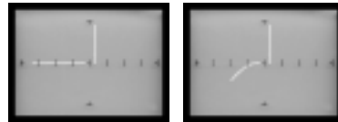
These signatures from good and bad comparator ICs show that damaged PN junctions are easily recognizable
