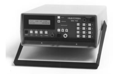
The Huntron DSI 700 adds digital storage capabilities to your Huntron Tracker 2000, making troubleshooting even easier than before. It quickly scans electronic components to determine the analog signature of each pin. These signatures can be used to compare a known good board with a questionable board for quick analysis.
